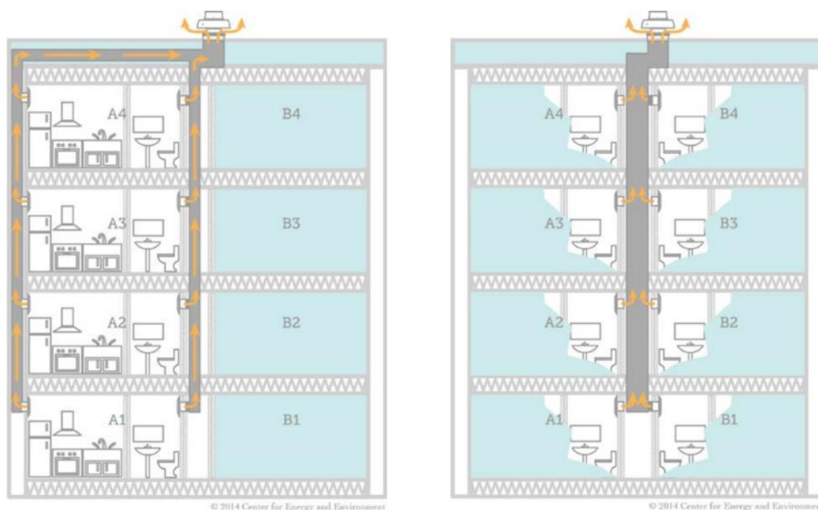
Figure 1 demonstrates the common centralized apartment exhaust fan configurations.
